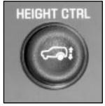
The button that controls this feature is located on the instrument panel to the right of the steering wheel.
